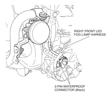
48. Secure the right front LED fog lamp harness with the wire tie as shown.
