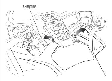
14. Insert the helmet holder into the gap as shown.Right side>
