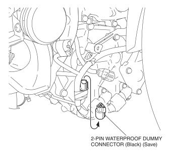
47. Connect the right front LED fog lamp harness as shown.
