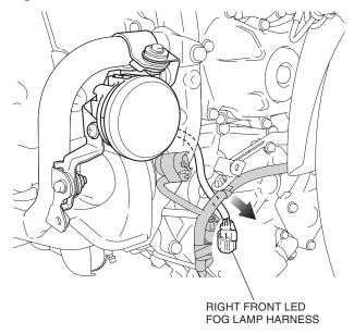
46. Remove the dummy connector as shown.
