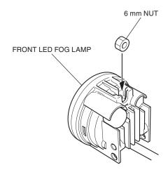
29. Loosely install the fog lamp adjust as shown. **<Left side>**
