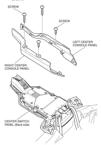
20. Remove the center console garnish as shown.
