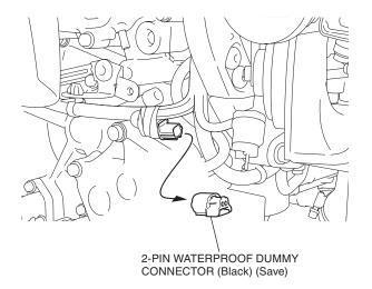
42. Connect the left front LED fog lamp harness as shown.
