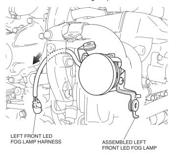
39. Install the assembled left front LED fog lamp as shown
