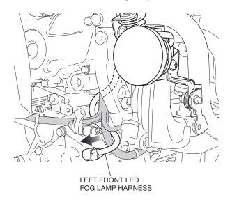
41. Remove the dummy connector as shown.
