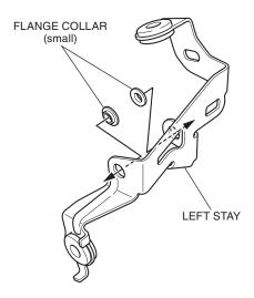
32. Loosely install the assembled left stay to the assembled front LED fog lamp as shown.
