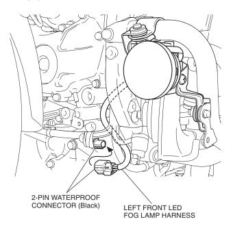
43. Secure the left front LED fog lamp harness with the wire tie as shown.
